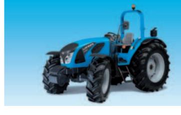
The 5H tractor range from Landini is revamped with the new Perkins 854E-E34TA 3.4L, four-cylinder engines, all featuring a two-valve cylinder head, a common rail injection system, turbocharging and an air-to-air aftercooling system. Equipped with an innovative exhaust gas recirculation system (EGR) which reduces NOx emissions at source, these engines meet the Tier 4 Interim emission regulations without the use of fuel additives.
