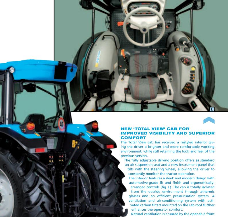
and rear windscreens, while a roof hatch provides extra visibility for loader work.
